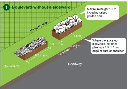
Where there are separated sidewalks (Figure 2), maintain a path of at least 50 cm along the curb edge to allow pedestrians to easily open and close vehicle doors, and to cross to the sidewalk from the street. Garden beds should be no longer than 6.0 m without a break of 1.0 m or more.
